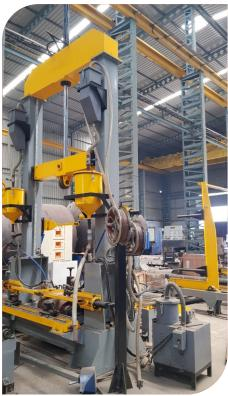
Elektra Vac Flux Recovery System have proven themselves as the most essential accessory to the entire Sub-Are Welding process. They save value of flux, helps make better welds and produce all important saving in man hours. Flux Recovery unit keep abrasive flux away from moving parts on the welding ring. These systems are capable of separating out slag and fine flux returning only the clean reusable flux to the hopper.
